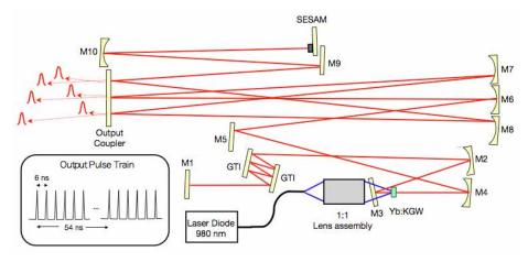
Fig. 2. Schematic representation of Yb:KGW oscillator layout. Mirrors are labeled by M1-M10, Gire-Tournois interferometer mirrors by GTI, and semiconductor saturable absorber mirror by SESAM. The laser cavity footprint is 125 cm by 50 cm.
