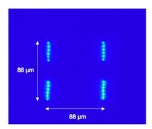
Fig. 4. Four corners of an 88  $\mu m$  by 88  $\mu m$  scan area for the six-foci system. Image shows overlaid CCD screen captures of two-photon fluorescence from Rhodamine-6G sample. Objective was a Zeiss A-plan 40×, 0.65 NA.
