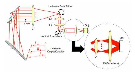
Fig. 3. Schematic representation of multifocal scan optics. Achromatic doublets are labeled L1-L5. Magnified inset shows beam configuration on back pupil of objective required for scanning. Central beams are omitted for clarity.
