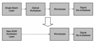
Fig. 1. Block diagram showing the simplification realized with the Yb:KGW multibeam laser design for nonlinear microscopy.
