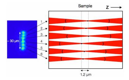
Fig. 5. Graphical portrayal of foci geometry in a sample. Axial dimension (z) is stretched relative to lateral dimension for clarity. The depth of focus is indicated by curved black lines on the focusing beam and the offset of the center of focus is marked by black dot. Beams are numbered top to bottom as arrayed in the CCD image capture.
